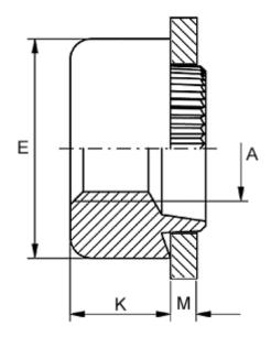
Female thread A = M5Height K = 4.0Outer diameter E = 9.0 Plate thickness = 3.2 to 3.4
